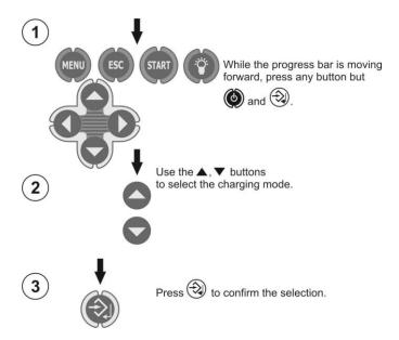
Charging the package of accumulators after a complete discharge is recommended if less than the normal number of measurements is possible to realise per charged package or in case of other doubts regarding the correctness of the displayed charge of the accumulators.
